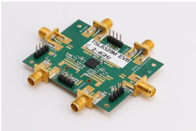
TagoreTech Front end module TSL8329M for TDD mMIMO applications, SW+LNA
